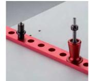
The drilling jig is moved and fixed wth the locating pin for longer rows of series drilled holes.
