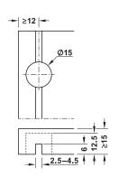
Application: The rear panel connector is pre-inserted into a drill hole in the groove and serves as a guiding and mounting aid for the rear panel. When the screw is tightened, the rear panel is pulled forwards and the connection reinforced
