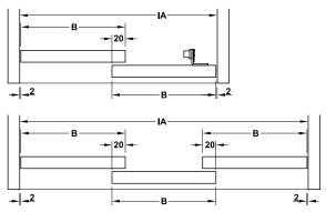
For 2 doors: Door width = (IA + 16)/2For 3 doors: Door width = (IA + 36)/3IA internal cabinet width, B door width
