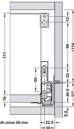
\* Min. dim. 49.5 mm, with Tipmatic Soft-close 58 mm
