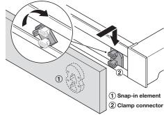
With large and heavy panels, the snap-in elements must be screwed or glued into the panel
