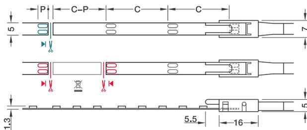
— Cut LED strip light to length (one contact side remains on the remainder piece; reusable)
