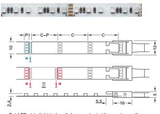
Cut LED strip light to length (one contact side remains on the remainder piece; reusable)
