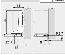
Set mounting plate back by glass thickness and height of cover cap +3 mm
