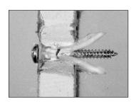
Positive tactile feedback of the setting key, in popping the anchor arms over center, is an absolute indication of proper hollow wall setting of the anchor. Do **not** place excessive pressure on the key and **never** use a hammer on it, since failure to set indicates either a solid wall or a wall too thick for the anchor to set in its hollow mode. The anchor **will** operate under such conditions, however, as a wedge and compression solid-wall anchor with significant holding strength.
