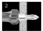
Insert anchor in hole and tap flush.
