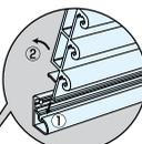
Install the bottom rail ①. Level the bottom rail before fastening. Insert the profile ② into the bottom rail. Fasten with screws.
