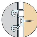
Install the profile ② until it reaches required height. The profile will cover the screws.
