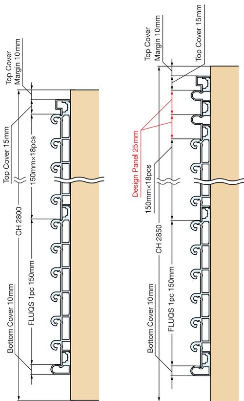
2 design panels are used to cover 50mm space in case of ceiling height 2850mm.
