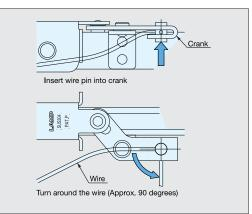
Installation of lock-release wire (WR and WL type only)
