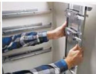
The main SERVO-DRIVE components can be attached without the need of tools
